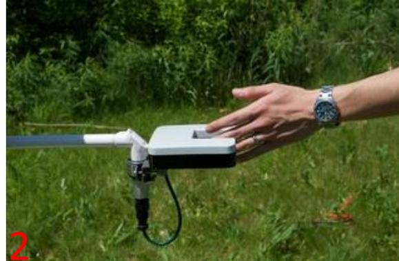
2 Trigger sensor by passing fingers through the opening 5 times.
