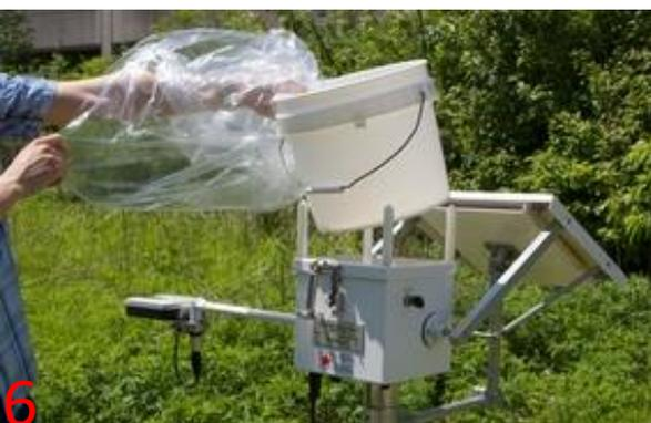
Turn power on to the collector, allowing it to close.
