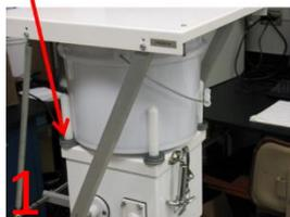
1 Select bucket to deploy from new, clean supplies. Note, washers may be needed to raise the bucket when it is deployed.
