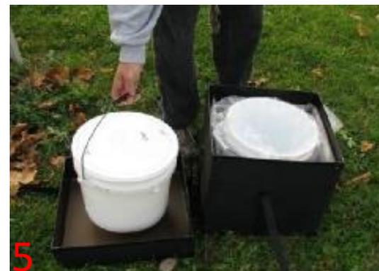
5 Remove sealed bucket from collector and set aside.
