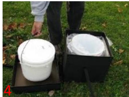
4 Remove sealed bucket from collector and set aside.
