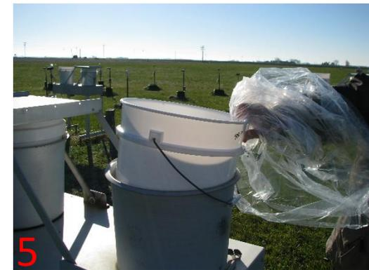
5 Deploy new, clean bucket using bucket bag as a glove.
