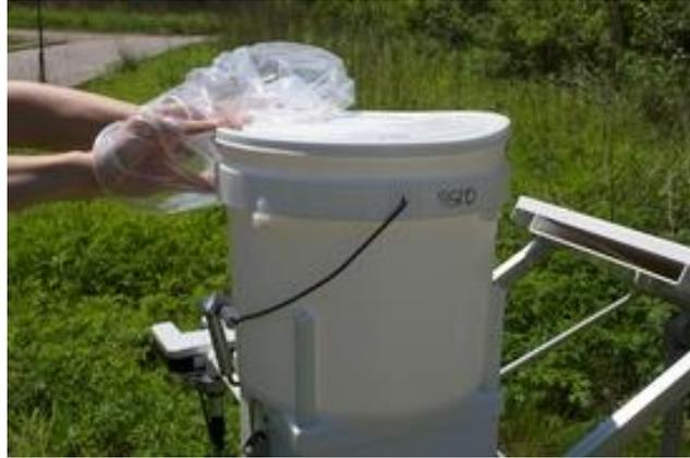
8. Lift the sealed bucket from the collector holder and place it in the carrier or on a clean surface. *Do not set the bucket on bare ground as dirt and dust are difficult to remove when the bucket is washed.* Verify that the lid is sealed firmly on the bucket.
