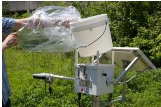
16. Using the switch on the bottom of the collector, turn the collector ON. The collector lid will close. The collector lid should move smoothly. Verify that the lid seal fits snugly over the bucket. If there is a gap between the bucket and the lid seal, it may be necessary to either:
