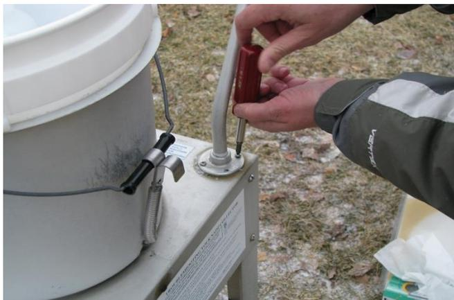
3. Remove the old sensor and set aside for return to the NADP Network Equipment Depot (NED).
