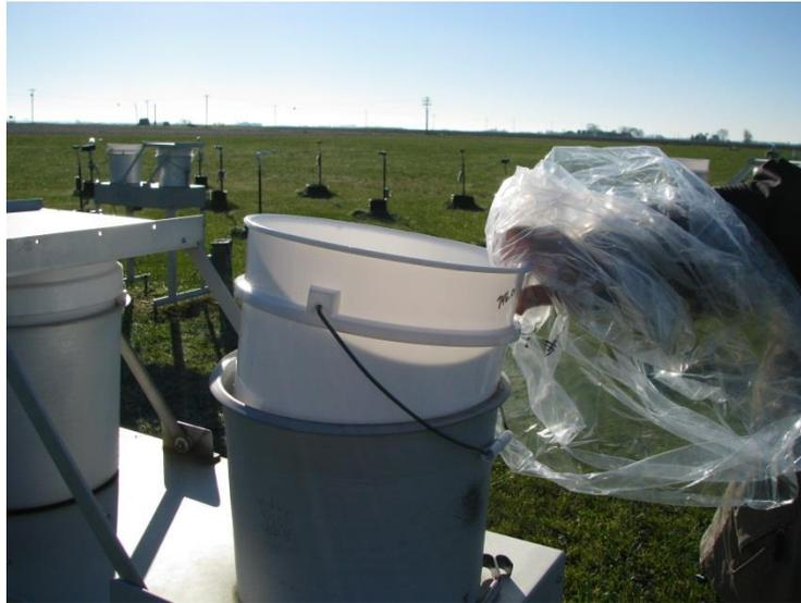
15. While face away from the sample bucket, blow across the surface of the grid sensor to remove excess water. This should help the collector close sooner. The collector lid should move smoothly. Verify that the lid seal fits snugly over the bucket.
