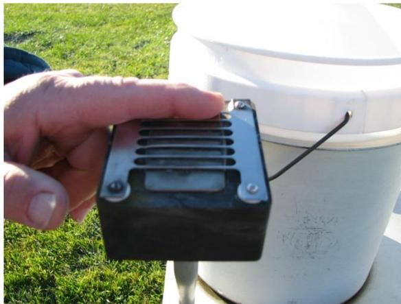
4. Activate the collector lid by placing several drops of water (DI, or tap), or a small amount of snow on the sensor. The collector should remain open for several minutes allowing change-out of the sample.
