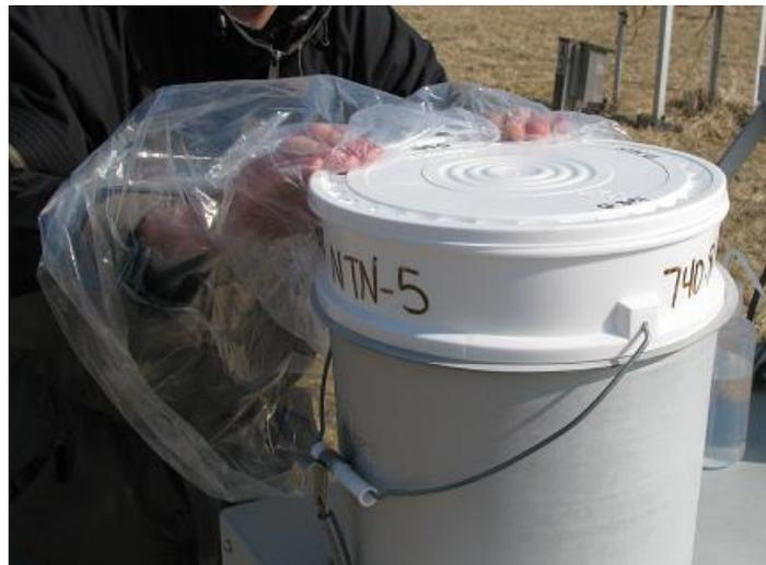
8. Lift the sealed bucket from the collector holder and place it in the carrier or on a clean surface. ***Do not set the bucket on bare ground as dirt and dust are difficult to remove when the bucket is washed.*** Verify that the lid is sealed firmly on the bucket.
