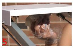
Wearing clean gloves, clean lid pad (with RO water) and collector surfaces (with 409).
