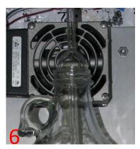
Wearing clean gloves, repeat steps 3 and 4 in reverse order to deploy new glassware. Ensure a good seal between the bulb and the bottle.
