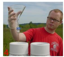
Remove used funnel and thistle tube. Remove blue clip. Re-bag glassware and place in MDN cooler.
