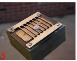
Trigger sensor with water/snow/ice.
