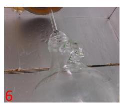
Wearing clean gloves, repeat steps 2 and 4 in reverse order to deploy new glassware. Ensure a good seal between the bulb and the bottle.
