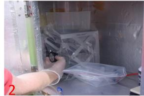
Lower jack. Wearing clean gloves, cap and bag the deployed sample bottle, and place in MDN cooler.
