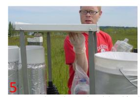
Wearing clean gloves, clean lid pad (with RO water) and collector surfaces (with 409). Replace dry-side bag.
