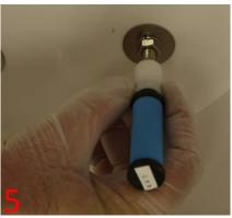
Wearing a new, clean glove, deploy the new sampler(s).
