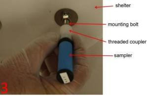
Wearing a clean glove (supplied), collect the deployed sampler(s) from the AMoN shelter. Return sampler to its glass jar and seal.
