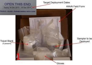
Inspect contents of AMoN supply box. Contact Site Liaison if jar(s) is/are cracked, or sampler(s) is/are broken.
