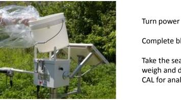
Deploy new, clean bucket using bucket bag as a glove.
