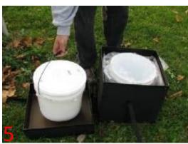
Remove sealed bucket from collector and set aside.
