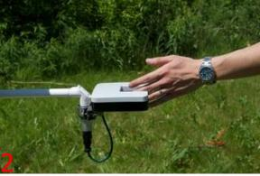
Trigger sensor by passing fingers through the opening 5 times. Turn off power to collector when it is open.
