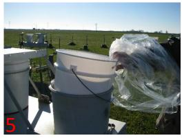
Deploy new, clean bucket using bucket bag as a glove.
