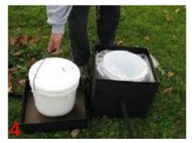
Remove sealed bucket from collector and set aside.
