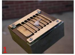
Trigger sensor with water/snow/ice.
