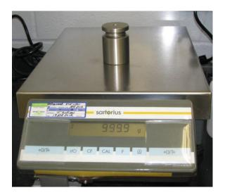
2. Weigh the sealed bucket containing last week's sample. Enter the mass (Bucket + Lid + Sample) in Block 6 **Bucket Sample Weight** of the FORF. Complete this step each week, regardless of whether precipitation occurred during the week. Network operating procedures require that the sample bucket be changed at least once every 194 hours (8 days and 2 hours).
