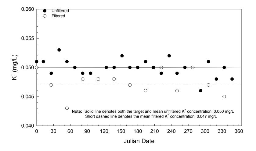
Figure B-4. Comparison of filtered and unfiltered internal blind samples, (potassium), High-Purity Standards, SR1, 1999.
