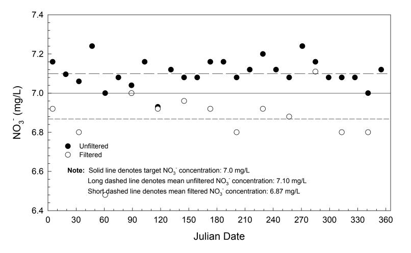
Figure B17. Comparison of filtered and unfiltered internal blind samples, (nitrate), High-Purity Standards, SR2, 1999.
