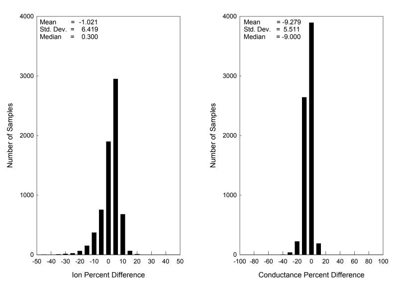
Figure V-1. Ion Percent Difference and Conductance Percent Difference for 6990 NADP/NTN wet samples, 1999.
