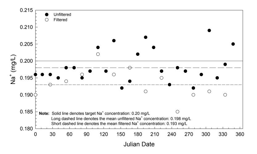
Figure B-3. Comparison of filtered and unfiltered internal blind samples (sodium), High-Purity Standards, SR1, 1999.
