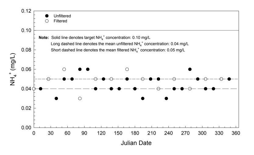
Figure B-5. Comparison of filtered and unfiltered internal blind samples, (ammonium), High-Purity Standards, SRI, 1999.
