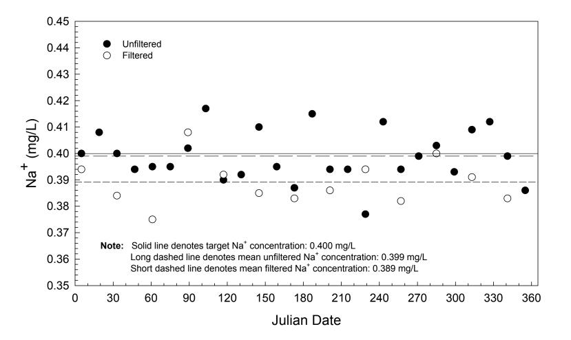
Figure B-13. Comparison of filtered and unfiltered internal blind samples, (sodium), High-Purity Standards, SR2, 1999.
