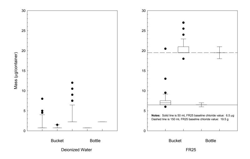
Figure B-38. Chloride found in upright bucket and 1-L bottle blanks using deionized water and FR25 QCS as leaching agents, 1999.
