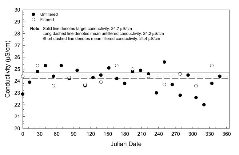
Figure B-10. Comparison of filtered and unfiltered internal blind samples, (conductivity), High-Purity Standards, SRI, 1999.
