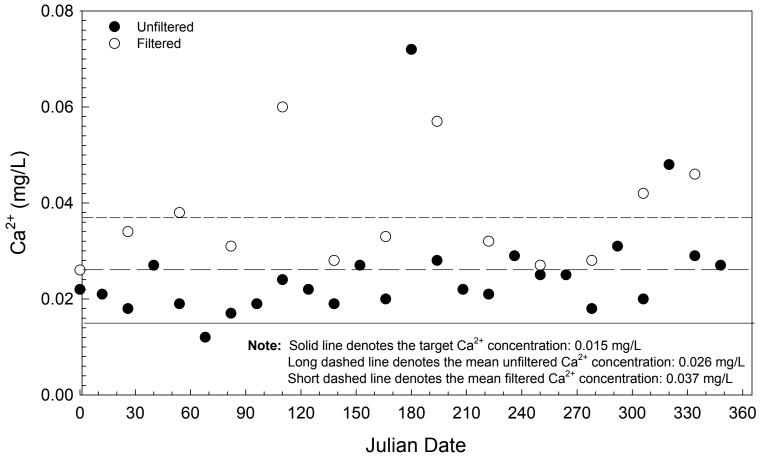
Figure B-1. Comparison of filtered and unfiltered internal blind samples, (calcium), High-Purity Standards, SR1, 1999.
