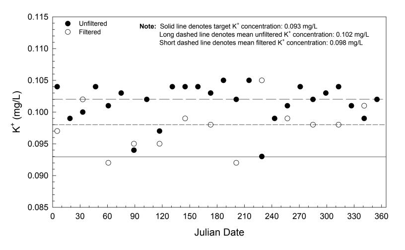
Figure B-14. Comparison of filtered and unfiltered blind samples, (potassium), High-Purity Standards, SR2, 1999.
