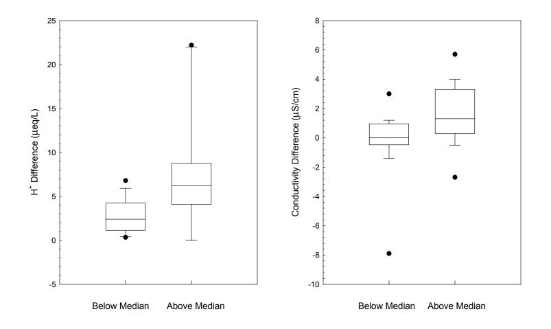
Figure B-28. Results of AIRMoN replicate analysis, hydrogen ion  $(H^{+})$  and conductivity, 1999.
