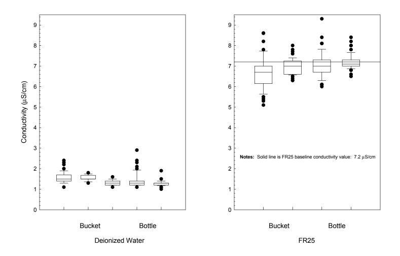
Figure B-40. Conductivity found in upright bucket and 1-L bottle blanks using deionized water and FR25 QCS as leaching agents, 1999.
