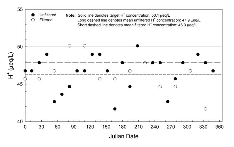
Figure B-22. Comparison of filtered and unfiltered internal blind samples (hydrogen ion), pH 4.3 nitric acid check sample, 1999.
