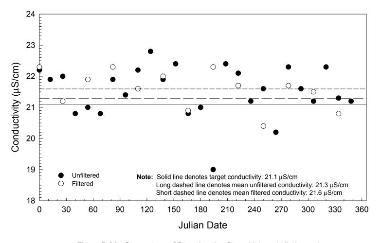
Figure B-23. Comparison of filtered and unfiltered internal blind samples (conductivity), pH 4.3 nitric acid check sample, 1999.
