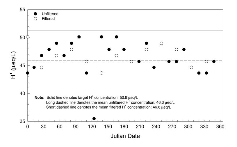
Figure B-9. Comparison of filtered and unfiltered internal blind samples, (hydrogen), High-Purity Standards, SRI, 1999.
