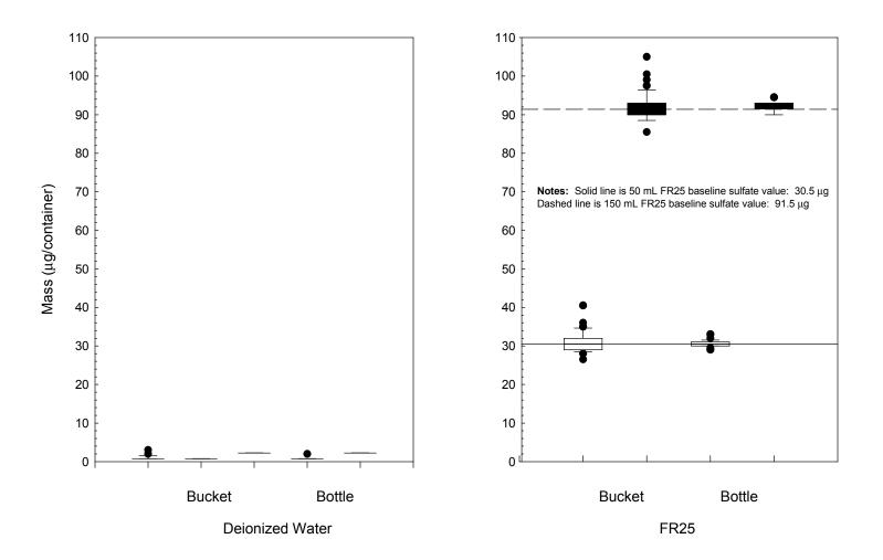
Figure B-36. Sulfate found in upright bucket and 1-L bottle blanks using deionized water and FR25 QCS as leaching agents, 1999.
