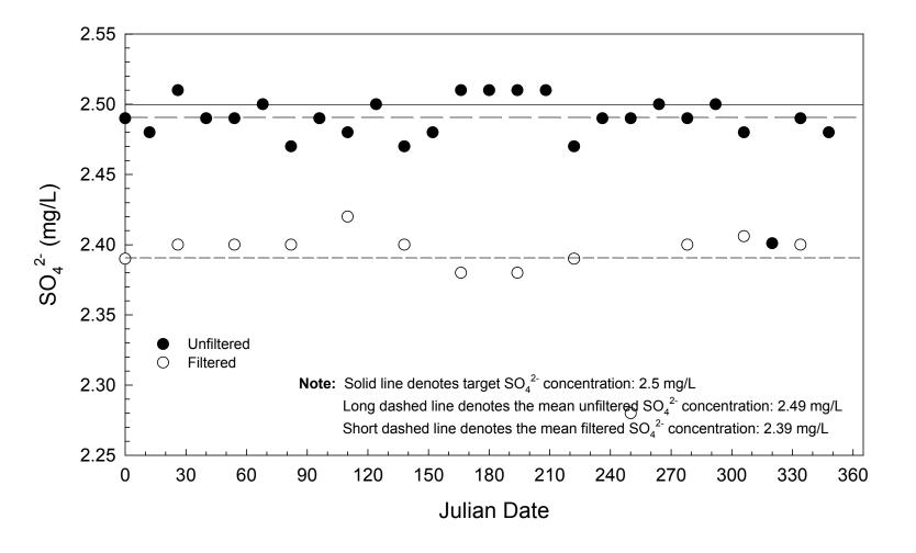
Figure B-6. Comparison of filtered and unfiltered internal blind samples, (sulfate), High-Purity Standards, SRI, 1999.
