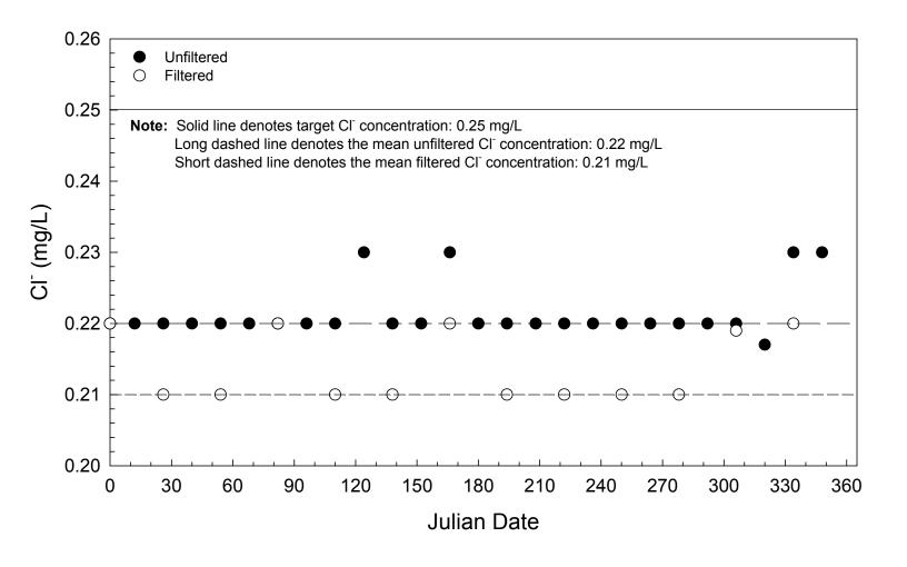
Figure B-8. Comparison of filtered and unfiltered internal blind samples, (chloride), High-Purity Standards, SRI, 1999.
