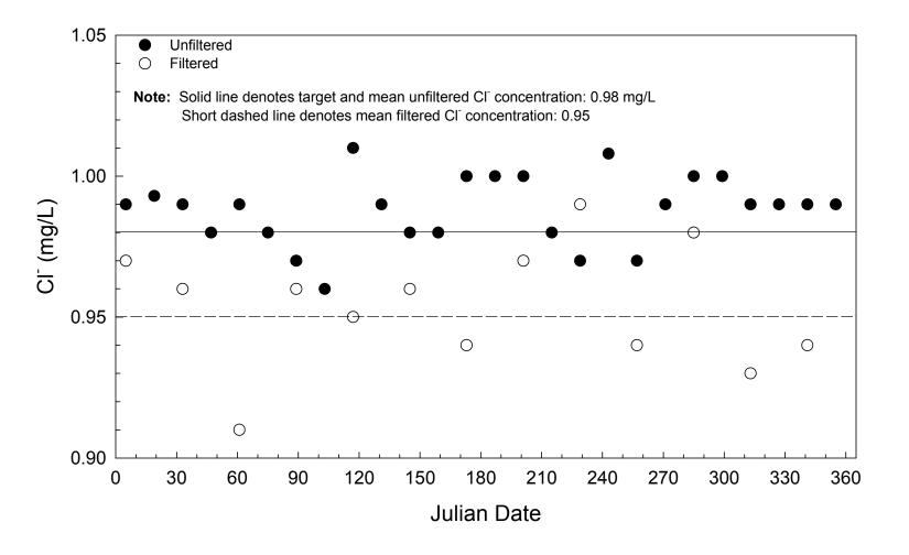
Figure B-18. Comparison of filtered and unfiltered internal blind samples, (chloride), High-Purity Standards, SR2, 1999.
