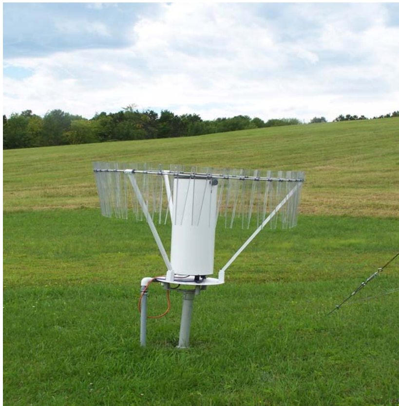
Figure 5-5. Gage Not Level – Not Stable – 45 Degree Rule Violation
