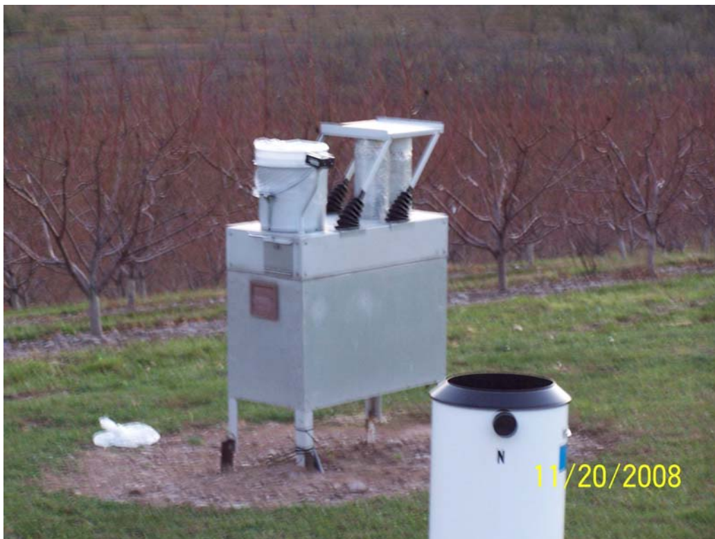
Figure 5-3. Optical Sensor Not Aligned North
