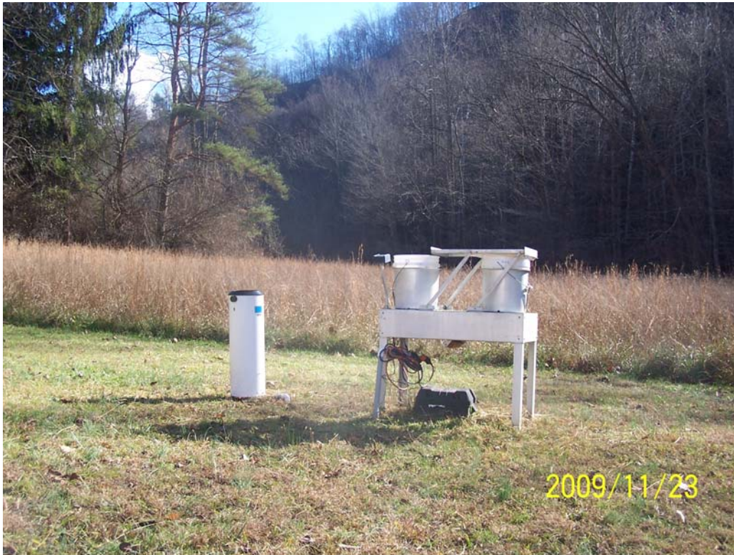
Figure 5-5. Gage Not Level – Not Stable – 45 Degree Rule Violation
