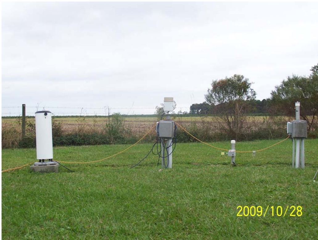
Figure 5-1. Power Cords Not Secured - Gage Not Level – Objects within 5 Meters
