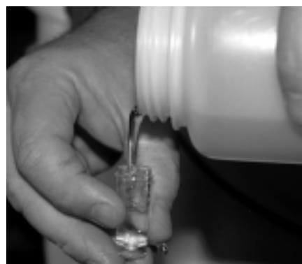
Figure 3-30. Rinse and fill four vials.
