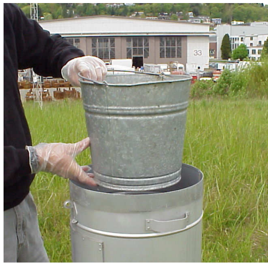
Removing the Belfort bucket.
