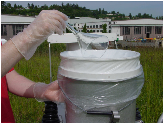
Removing old dry-side bag.
