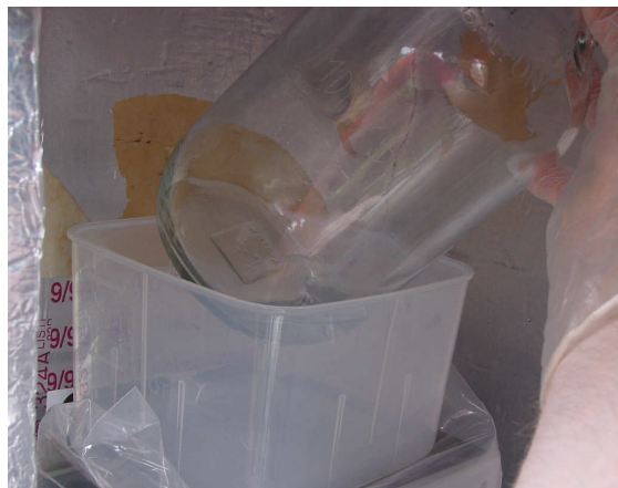
Placing new sample bottle in overflow dish.
