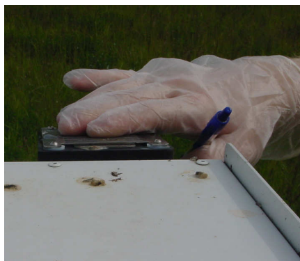
Feeling if the sensor is heating properly.
