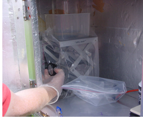
Lowering jack to gain access to sample bottle.
