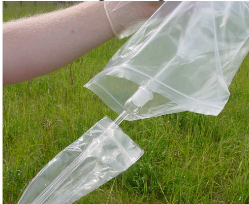
Connecting funnel and thistle tube using clean sample handling.
