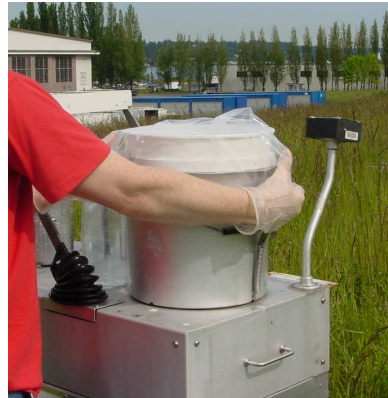
Securing new dry-side bag.
