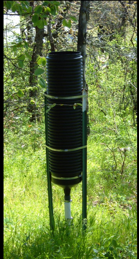
ion resin exchange column with snow tube
