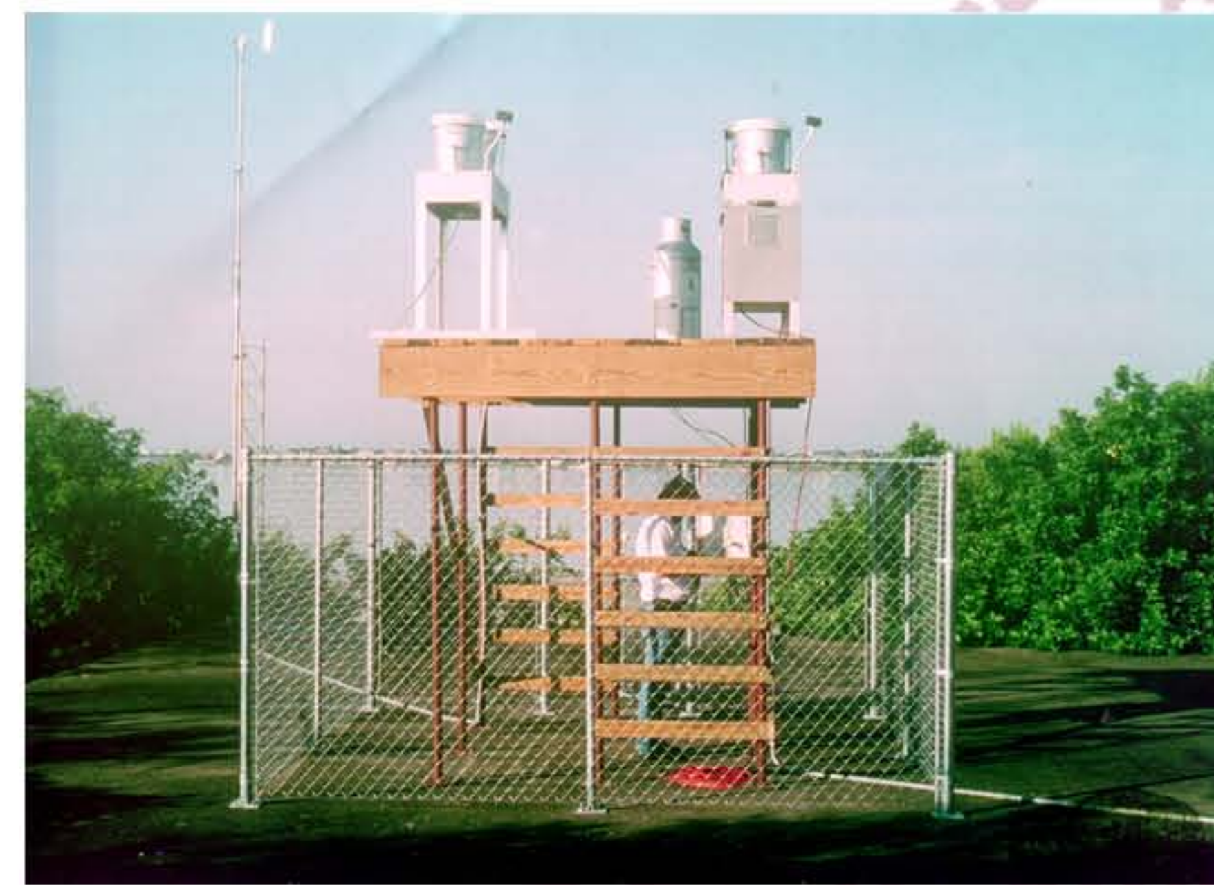
Figure 2. TAMUCC Station, note AeroChometrics wet-dry samplers and the Belfort rain gauge in the foreground and the meteorological sensors in the background.
