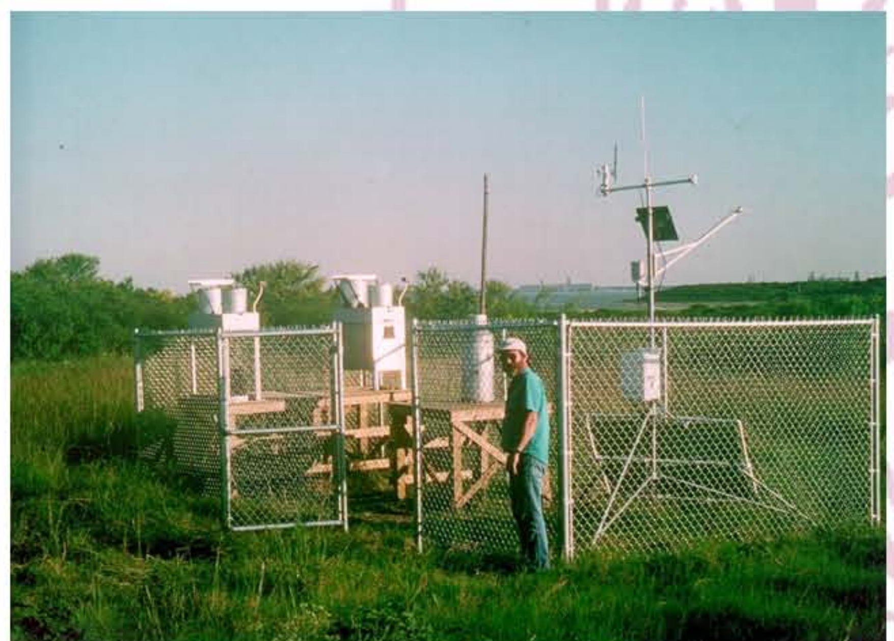
Figure 3. Whites Point Station, note the meteorological sensors and the Belfort rain gauge in the foreground, the AeroChometrics wet-dry samplers in the background, industrial complex on the horizon.
