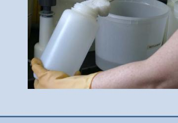
The NTN & AIRMoN use 3.5 gallon HDPE buckets to collect precipitation samples. In the NTN, these buckets are exposed to field conditions for one week. Buckets are washed with deionized water at the CAL and reused. Four blanks are prepared weekly from randomly-selected buckets. Solutions include:
