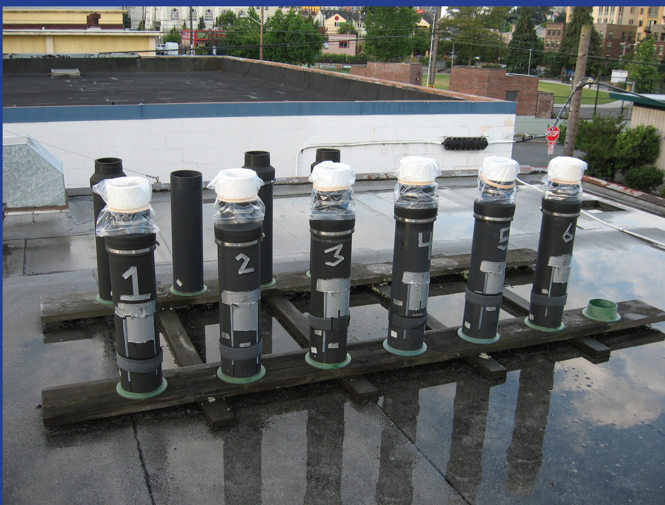
Figure 1: Sample collection shells with covered funnels
