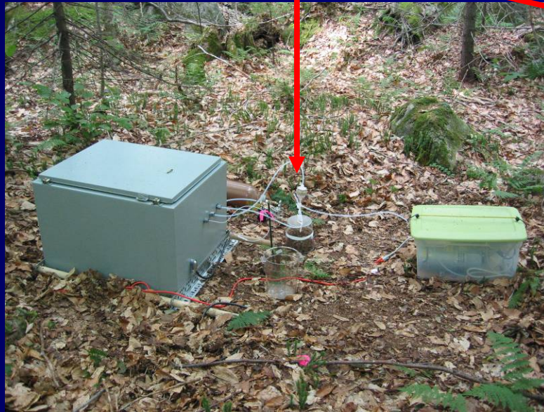
DFC operation system for measuring Hg emission flux from soils
